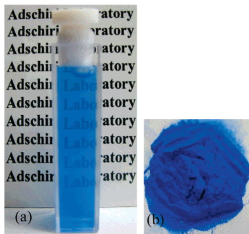
Figure 1. (a) Dispersion of oleic acid capped cobalt blue nanocrystals pigment in hexane (1 wt %); (b) cobalt blue nano pigment powder.
